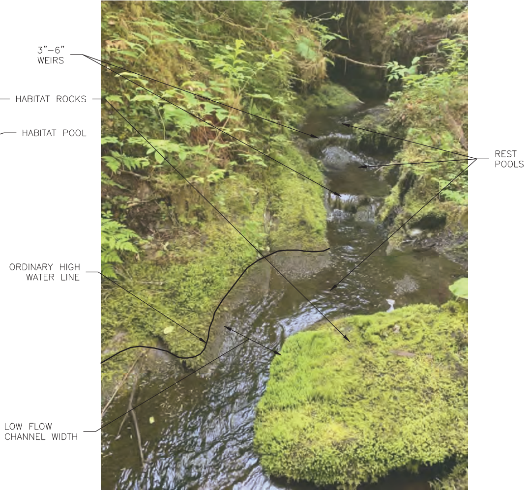
2 EXAMPLE REACH - WEIR SECTION J5.0 > 2.0%
